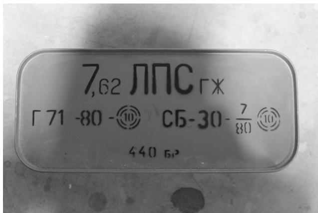
Figure 3.8 A sealed tin containing 440 7.62×54mm cartridges produced by Arsenal Bulgaria. The twin circles surrounding the number 10 indicate the manufacturer; the second number in the sequence, left of the manufacturer identification, is the production year. The caliber is identified at the top and the number of pieces on the bottom. Soviet-era military ammunition is similarly packaged and marked. (Image from author's collection.)
